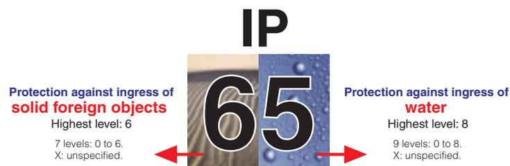
The International Electrotechnical Commission standard IEC 60529 describes a system for classifying degrees of protection provided by enclosures of electrical equipment. The IP Code consists of the letters IP and two numerals. Larger numbers represent greater levels of protection.
