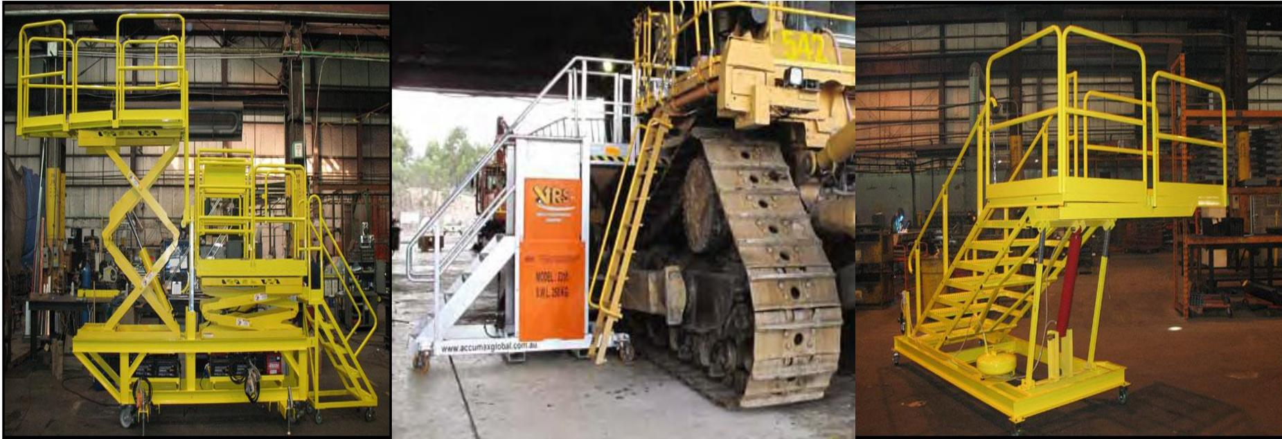
Adjustable height platforms provide the ability to operate at a wide range of platform heights. These platforms provide the user access to various working positions.
