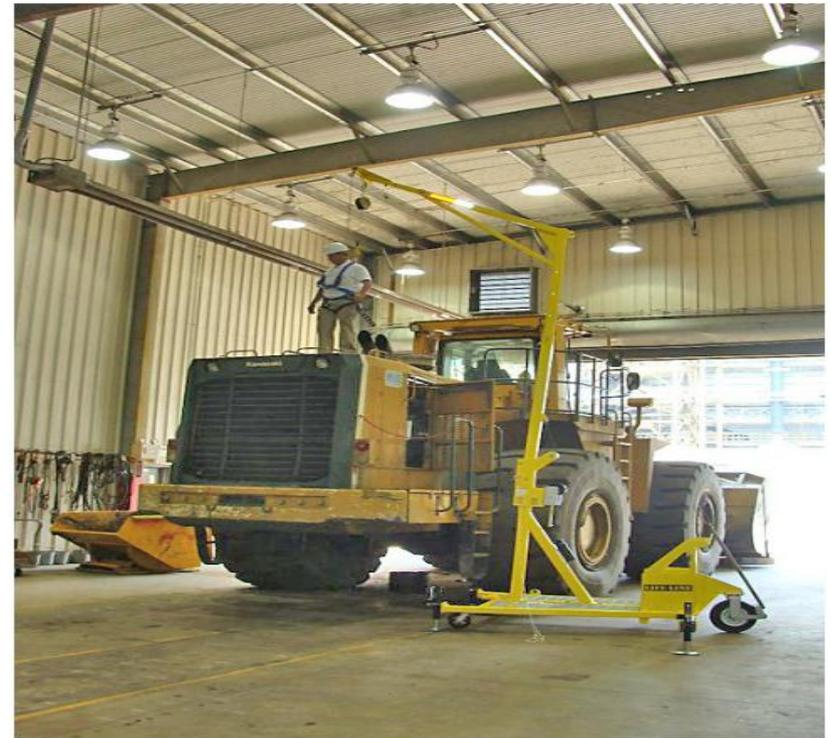
For work environments where an overhead anchor point is not possible and clearance is limited, Mobile Single Point Anchors (MSPA) from Flexible Lifeline Systems® provide safe access for working surfaces. The system features models with adjustable anchor point heights of up to 22 feet, as well as outriggers that enlarge the base foot print to stabilize and level the system when in use
