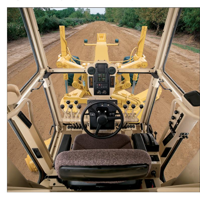
**Exceptional visibility** helps improve operator confidence and productivity in all grader applications. The large front glass area provides an unobstructed view of the moldboard and front tires. The large side windows offer a clear view of the moldboard heel and tandem tires. A wide rear window and tapered engine hood provide good visibility to the rear of the machine, especially to a rear ripper.
