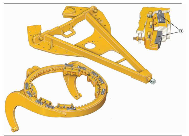
Rugged construction. The drawbar features an A-frame, box-section design for high strength. The bottom is machined to provide accurate adjustment and precise blading. A one-piece forged circle is built to stand up to high stress loads. To resist wear, teeth are induction-hardened in the critical areas. For maximum support, the circle is secured to the drawbar by six support shoes.
