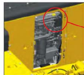
Electric priming pump switch
