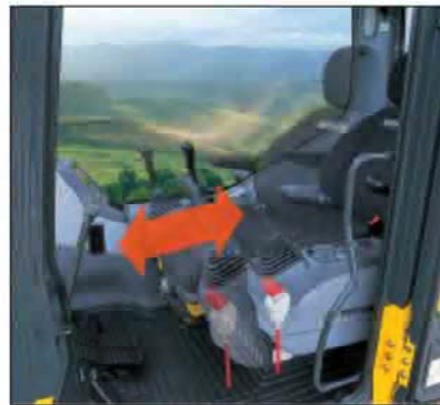
Seat Sliding Amount: 340 mm 13.4", increased 120 mm 4.7"
