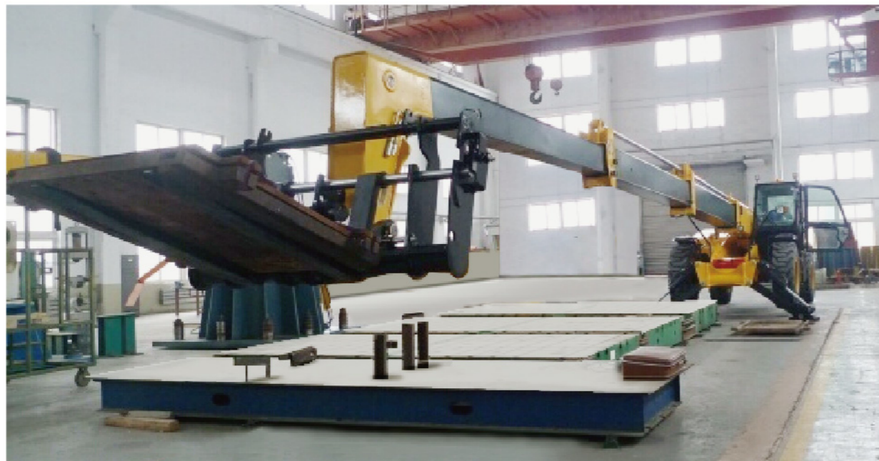
XC6-4517叉装机通过20万次疲劳载荷及超载试验 XC6-4517 has passed fatigue load and overload tests of 200,000 times
