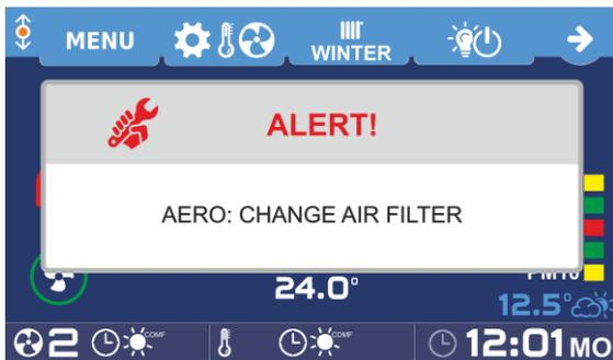
2. DIRTY FILTER! text flashing on the VENTILATION INFO screen.
