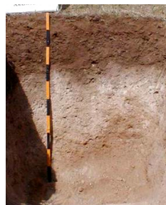
Fig. 1 Picture of soil profile at JGH for example. White colored horizon is the Bk horizon.
