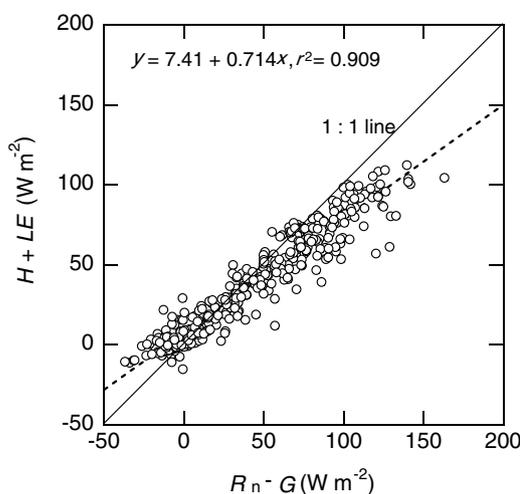
**Figure 1** Test of energy balance closure: the daily sums of sensible ( $H$ ) and latent heat fluxes ( $LE$ ) are plotted against the daily differences between net radiation ( $R_n$ ) and soil heat flux ( $G$ ).
