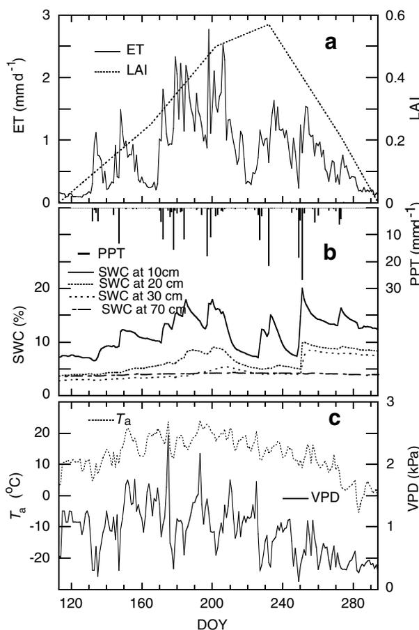
**Figure 3** Temporal variation of (a) daily evapotranspiration rate (ET) and leaf area index (LAI), (b) daily precipitation (PPT) and daily mean soil water content (SWC) at depths of 10, 20, 30 and 70 cm, and (c) daily mean air temperature ( $T_a$ ) and corresponding atmospheric vapor pressure deficit (VPD) during the growing season.
