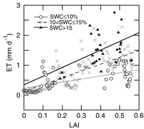
**Figure 5** The relationship between daily evapotranspiration rate (ET) and leaf area index (LAI) during the growing season. The data were compiled into three classes of soil water content (SWC) at 10 cm and each class was fitted to a linear function ( $ET = b_0 + b_1 \times LAI$ ):
