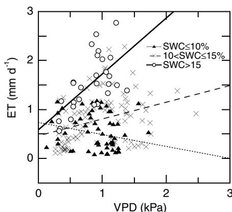
**Figure 6** The relationship between daily evapotranspiration rate (ET) and daily mean vapor pressure deficit (VPD) during the growing season. The data were compiled into three classes of soil water content (SWC) and each class was fitted to a linear function ( $ET = c_0 + c_1 \times VPD$ ):
