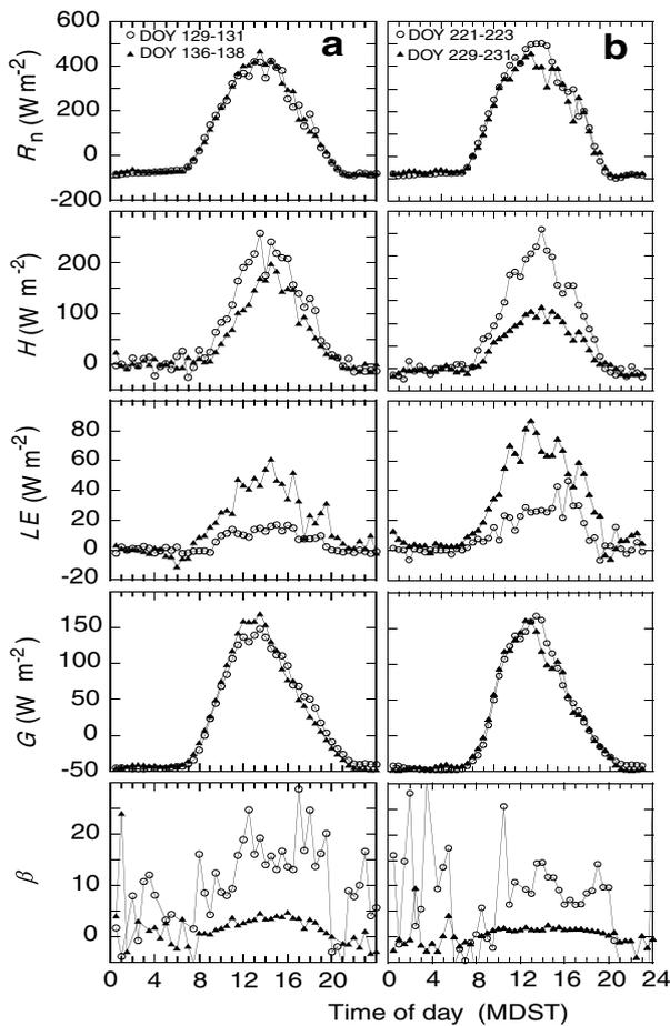
**Figure 2** Three day ensemble half-hourly average of net radiation ( $R_n$ ) and its partitioning between sensible ( $H$ ), latent ( $LE$ ) and soil heat flux ( $G$ ) as a function of time of day prior to (open circles) and immediately after (solid triangles) the precipitation event: (a) Stage I, and (b) Stage II. Time of day is Mongolian Daylight-saving Standard Time (MDST). The time difference between MDST and local solar time is 1.8 h. Data are summarized in Table 1.
