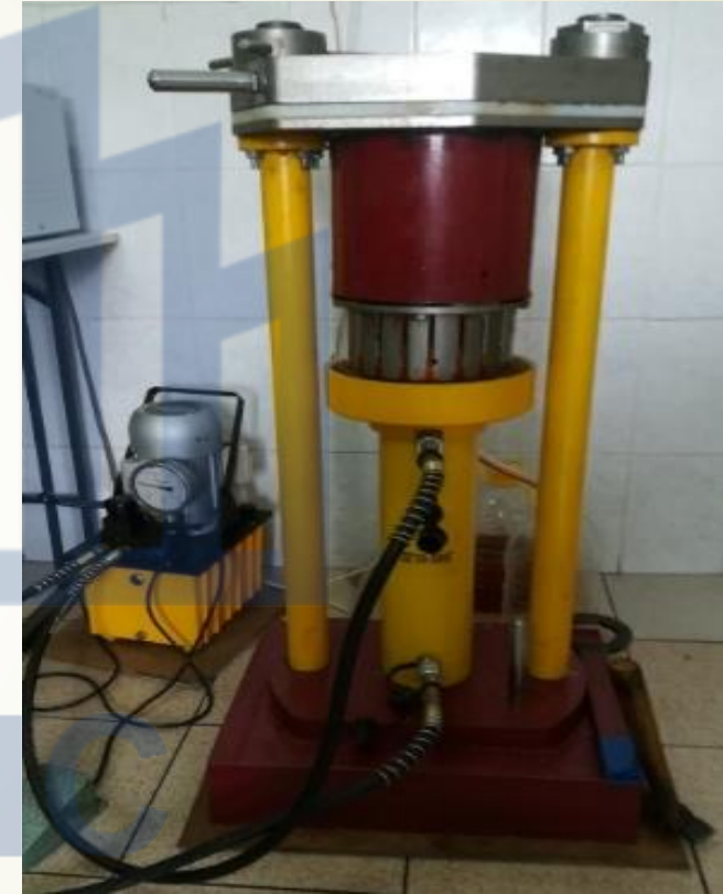
Authors and designed for pressing fresh or dried sea buckthorn fruits to produce sea buckthorn oil or juice
