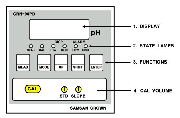
3-1 Display : display of measured value, set-value, parameter's set contents
