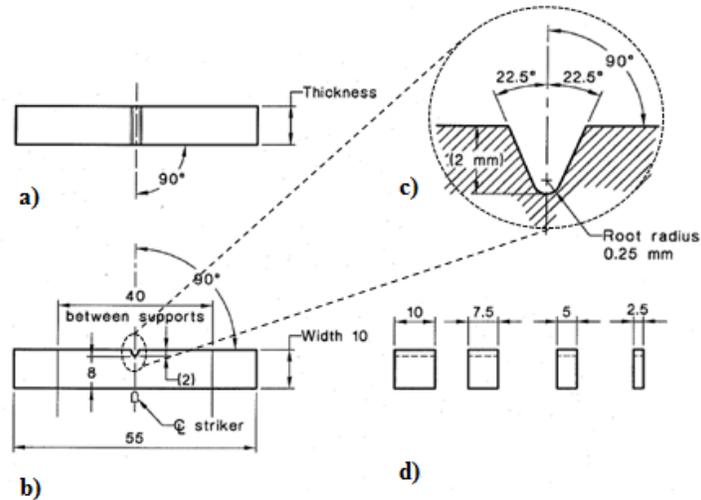
Figure 1. CVN specimen: (a) top view; (b) side view; (c) Notch detail; (d) Subsidiary specimens
