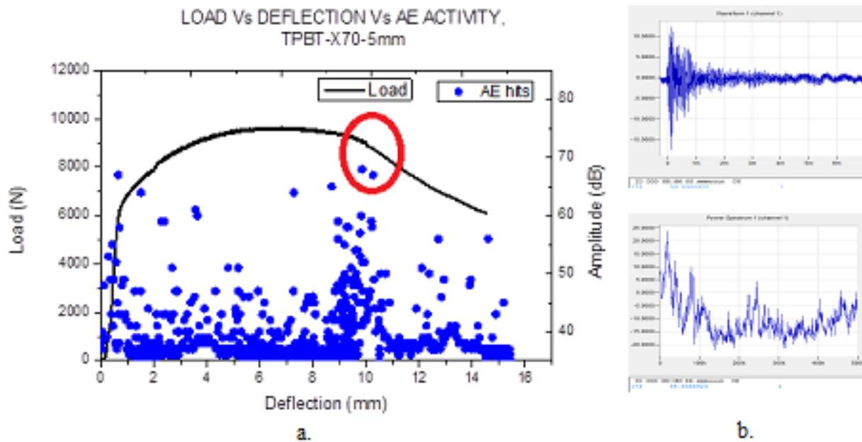
Figure 4. The AE activity corresponding to the load-deflection curve obtained during testing of three point bending test (a) and its selected AE signal waveform and power spectra (b) corresponding to fracture initiation for CVN specimen with 5 mm thickness.
