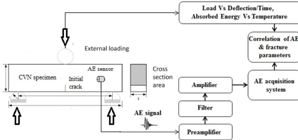
Figure 2. The schematic experiment setup of the TPBT
