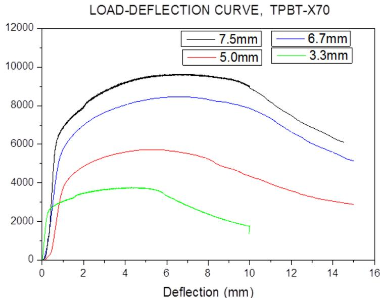
Figure 3. Typical Load-Deflection curve for TPB test at ambient temperature of specimens with various thicknesses.
