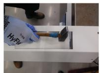
Remove the pre-cut part with a hammer.
