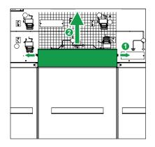
To remove the cover, remove the 2 screws on each side of the cover then lift it and pull it towards you. The instructions are visible on the cover.
