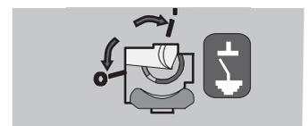
Switch or circuit-breaker closed: the earthing switch is blocked.
