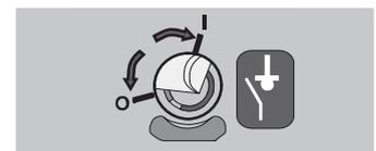
Earthing switch closed: the switch or circuit-breaker is blocked.
