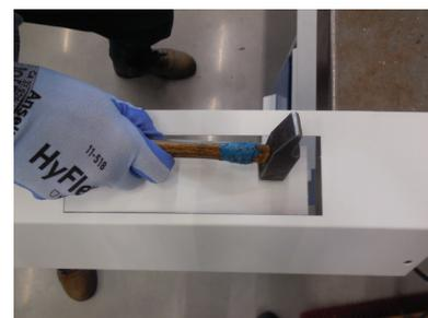
■ Remove the pre-cut part with a hammer.
