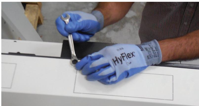
■ Disassemble the duct cover. Remove the 6 screws using a wrench.
